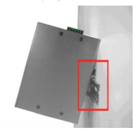
Step 2: Push the switch toward the DIN-Rail until you hear the spring snap into place
