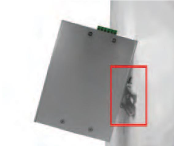
Step 2: Push the switch toward the DIN-Rail until you hear the spring snap into place
