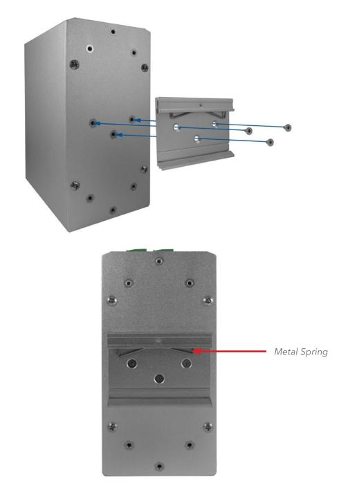
Each switch has a Din-Rail kit on the rear panel. The DIN-Rail kit affixes the switch to the DIN-Rail. It is easy to install the switch on the Din-Rail:
