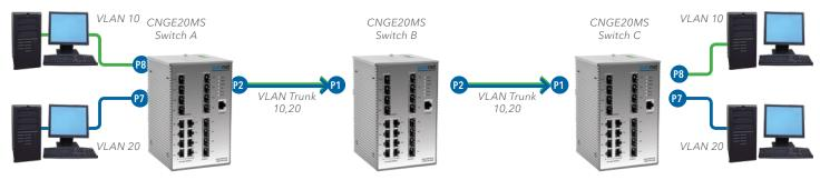
In the topology above, for Switch A, Port 7 is VLAN Access mode = Untagged 20 Port 8 is VLAN Access mode = Untagged 10
