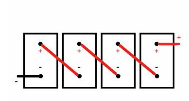
Connect the unterminated end of the Negative wire to port 3 on the controller
