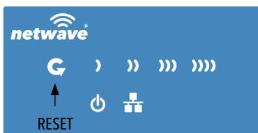
Press and hold the reset button for 4-30 Seconds to reset the radio back to factory defaults.
