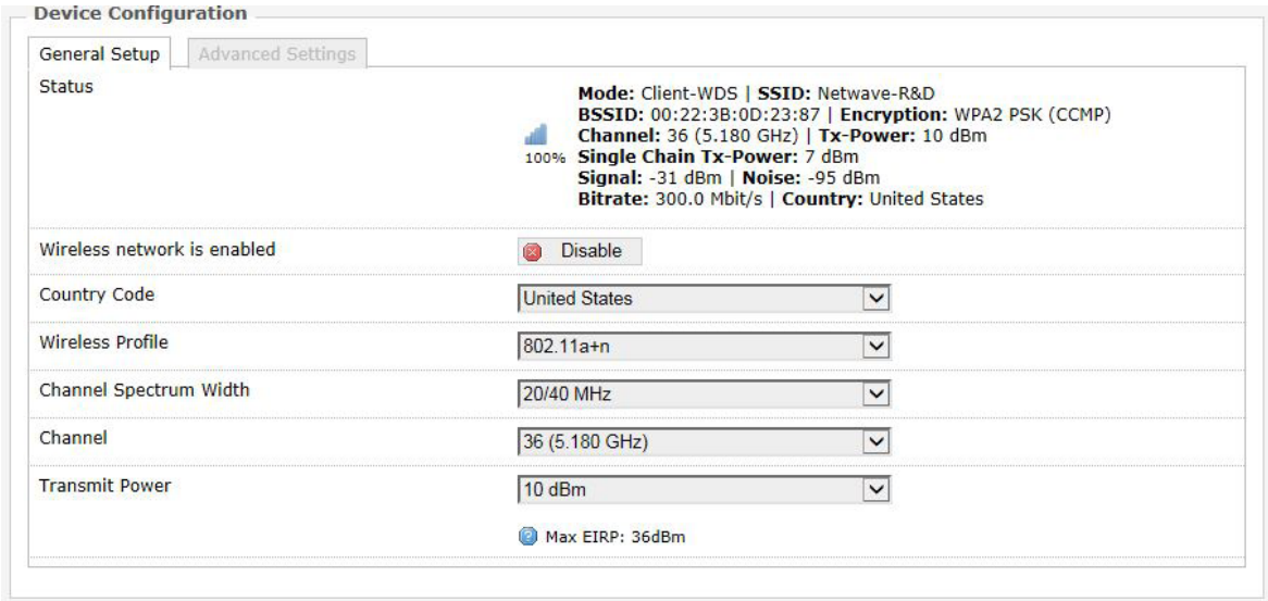
Figure 40: The WiFi Device Configuration section.
