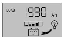
**Cumulative Load Discharging Ah** The displayed number is the cumulative discharging Ah of loads. To clear the figure and begin a new count, press and hold the
