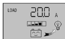
**Load Current** The displayed number is the load current.
