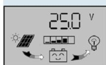
**Battery Voltage** The displayed number is the current battery voltage. This is the main interface, and shows the charging and discharging state, battery capacity and battery voltage.
