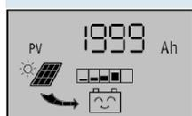
**Cumulative Generating Ah of Solar Panels** The displayed number is the cumulative generating Ah of the solar panels. To clear the figure and begin a new count, press and hold the
