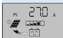
**Generating Current of Solar Panels** The displayed number is the generating current passing through the controller from the solar panels.
