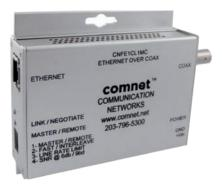
in VDSL (Very high-speed Digital Subscriber Line) technology. One is a modem unit that allows the use of Ethernet over a conventional copper twisted pair circuit, up to a maximum of 3km (9,800ft) between modems, making it ideal for Ethernet-based signalization systems. The other is a modem unit that allows the use of Ethernet over conventional  $75\Omega$  coaxial cable, up to 2.6km (8,500ft).
