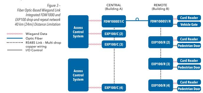
Up to 8 EXP100s can be daisy-chained together per channel (see figure 3) to easily and effectively create a Wiegand, Magstripe, or F/2F-based drop-and-repeat/daisy-chain topology, and each EXP100 may be set to a unique address (1 thru 15) via DIP-switch selection. Only one DIP-switch is required to be set at time of installation. The EXP100 series are supplied as a remote unit (ComNet model EXP100/R) for door or gate locations, and a central unit (model EXP100/C) for control panel installation.
