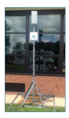
To get the video back to the head-end monitoring location, the ComNet NetWave NW1 point to multipoint models were selected. The four NW1 client units were installed close to the camera locations. The camera output was 10 frames per second at 1280 × 720 resolution. Using H.264 compression, each of the four cameras required 2.5Mbps of bandwidth. The Netwave NW1 handles up to 95Mbps, so the total 10Mbps bandwidth from
