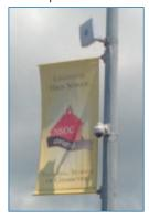
all came up without any trouble. Four Pelco IM Surevision 1.2 Megapixel day/night AF Low Light WDR Rugged Cameras were placed at strategic locations, the furthest being 90 yards away from the monitoring location. Two cameras were observing the backside of the wall and two more were observing activity from the front. This setup gave complete coverage of the entire event.
