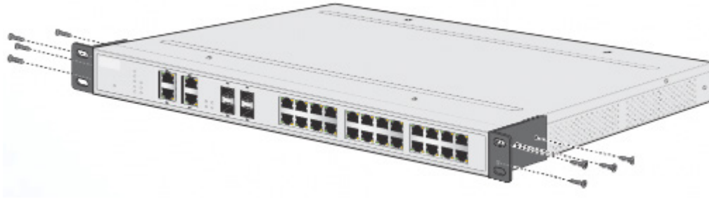
Figure 2-1. Installing the Rack Mount Brackets
