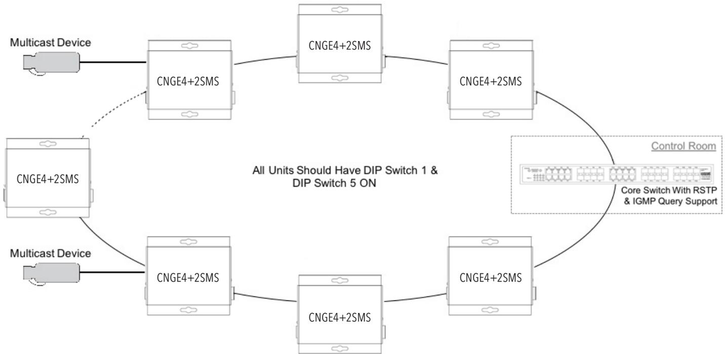
**Important Note:** The CNGE4+2SMS supports IGMP snooping only. When using the IGMP function a managed switch must be implemented within the network that is configured as the IGMP Querier as shown. Up to 64 IGMP groups are supported on the CNGE4+2SMS switch.
