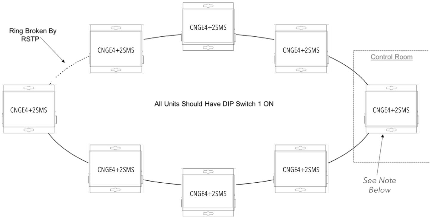
**Attention:** ComNet recommends maximum number of units per ring is limited to 20 devices. Numbers higher than this may cause undesired performance and are not supported by ComNet.
