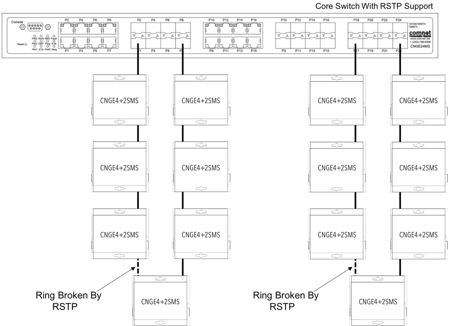
**Attention:** ComNet recommends maximum number of units per ring is limited to 20 devices. Numbers higher than this may cause undesired performance and are not supported by ComNet.
