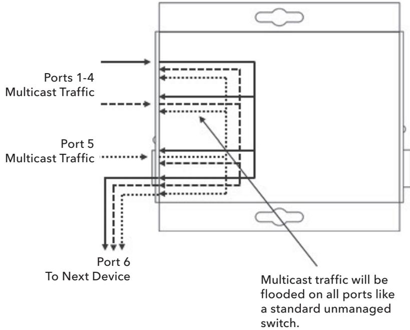
SMS MUX Enabled (DIP Switch 3 in ON Position)
