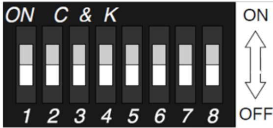
DIP Switches 6, 7, and 8 set the number of expansion module pairs.
