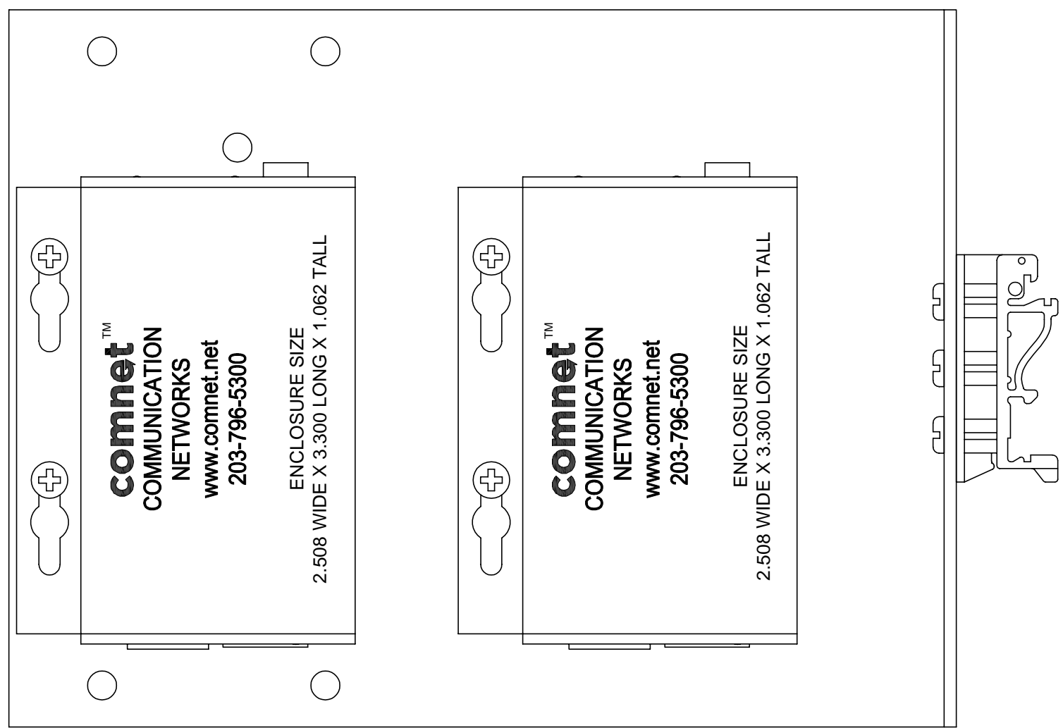
COMNET "MINI-LONG SIZE" MODULE IN VERTICAL POSITION USE HOLES CODED "D", "E", "L" AND "M"
